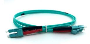
The duplex fiber patch cord is OM3 with 3 mm jacket. It is LSZH rated and its terminated with LC fiber optic connector on both ends.
